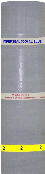
**IMPERSEAL 3000 XL BLUE** is a tough preformed waterproofing membrane comprising a strong cross laminated multi layer HDPE film with superior mechanical properties and a thick elastic self adhesive SBS/ Bitumen compound, designed to provide sub-structure concrete surfaces with high waterproofing protection.
